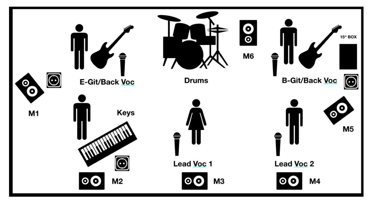
KEYS: OUTPUT: 2 x 6,3mm JACK DIRECTLY INTO P.A. via D.I.BOX
